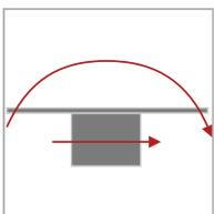
Sound reduction in ceiling construction, no mineral wool backing, **non-perforated tile**, 200 mm suspension 35 dB  $D_{n,f,w}$
