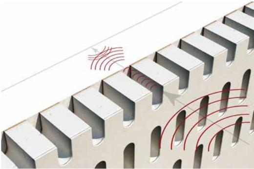
Knauf Danoline acoustic ceilings absorb the sound waves in three ways: by the vibrations of the acoustical tiles, by the resonance created in the perforation holes and by the acoustic felt backing.
