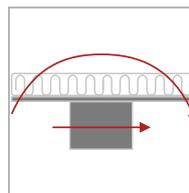
Sound reduction in ceiling construction, 50 mm mineral wool backing, **perforated tile**, 200 mm suspension 41 dB  $D_{n,f,w}$
