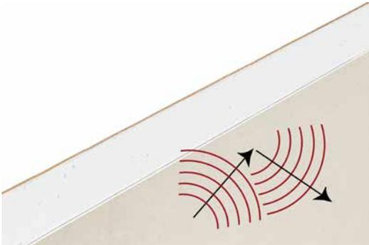
Due to the hardness of the gypsum tile, it is also able to reflect some of the sound waves in the room. These waves are reflected by the non-perforated parts of the tile, the perimeter border around the perforated area in particular.
