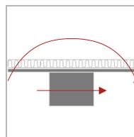
Sound reduction in ceiling construction, 25 mm mineral wool backing, **perforated tile**, 200 mm suspension 36 dB  $D_{n,f,w}$
