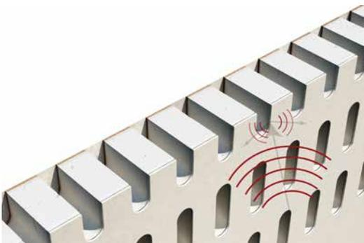
In addition to absorbing the sound waves, the perforation holes in a gypsum tile also create sound diffusion. The sound diffusion is enabled thanks to the complex structure of the perforated tile, contrary to e.g. a non-perforated gypsum tile or a fibrous absorber.
