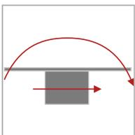
Sound reduction in ceiling construction, no mineral wool backing, **perforated tile**, 200 mm suspension 23 dB  $D_{n,f,w}$
